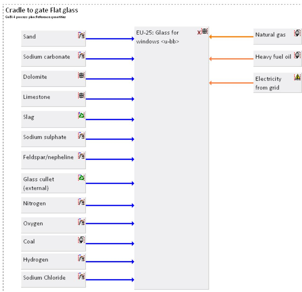
Figure 1: Cradle-to-gate system model of float glass
